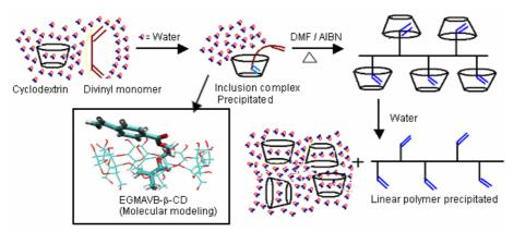
In the methodology developed at NCL / IICT. the water insoluble divinyl monomers form an inclusion complex β-cvclodextrin with and its derivatives such as dimethyl Bcyclodextrin. The vinyl group included in the cavity of  $\beta$ cvclodextrin does
